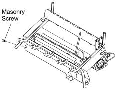
Figure 12 - Attaching Heater to Fireplace Floor
